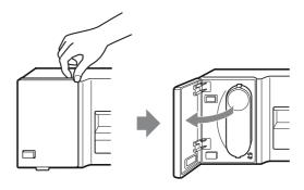
Remove the ink ribbon cassette by pressing the EJECT button.
